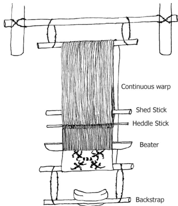
Illustration 2: The basic components of a backstrap loom.
