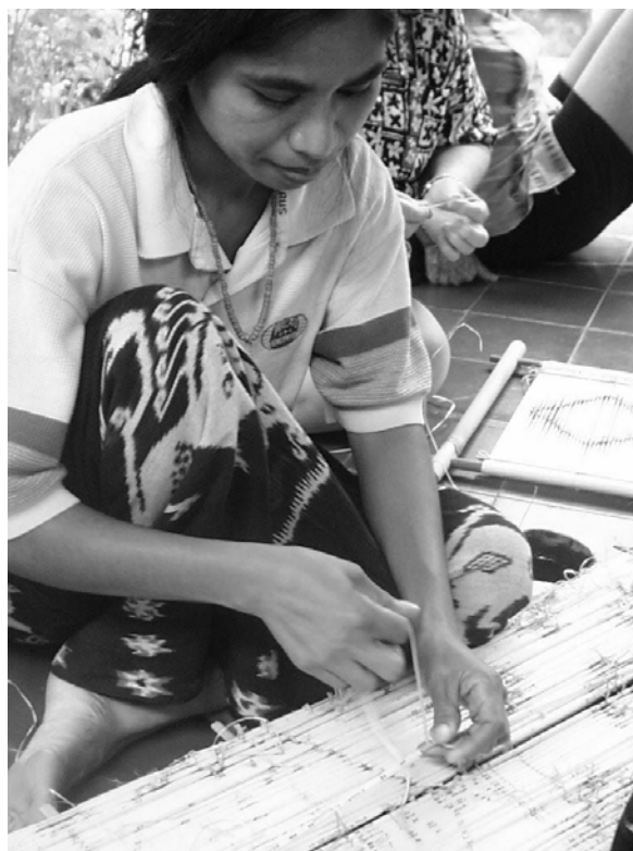
Illustration 7: Imelda Ndwa tying warp threads to a pattern ready for dyeing (Ikat). The damp tying fibre makes a squeaking noise as she tightens each knot. Karen Madigan 2004
