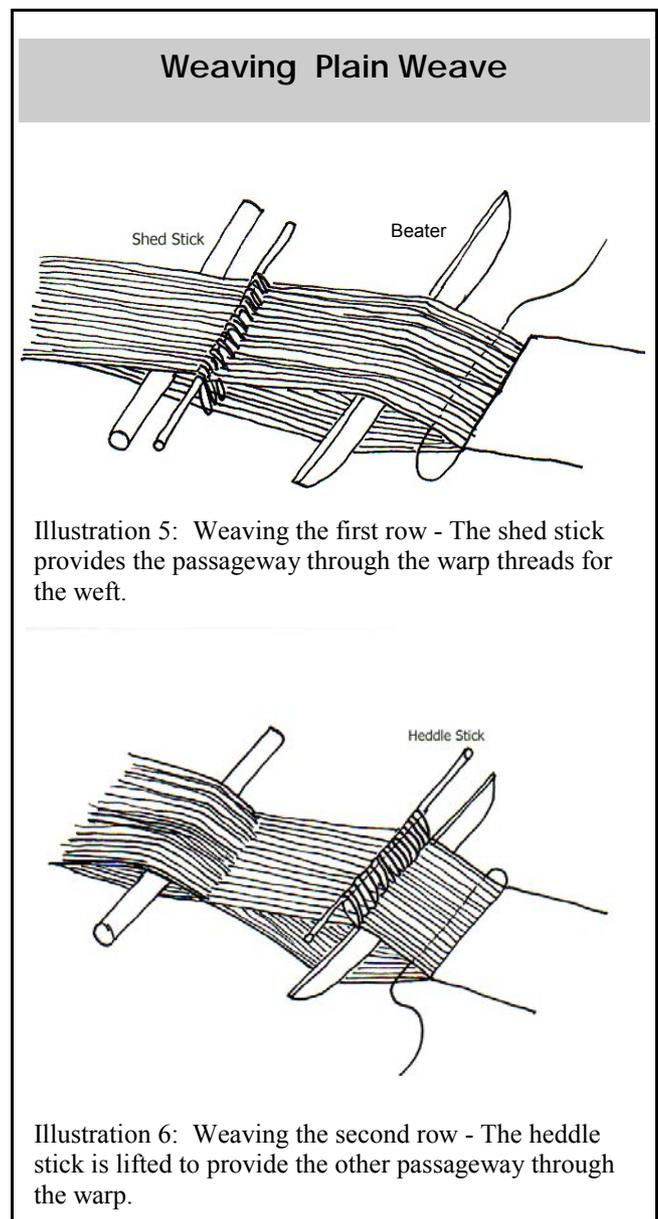
Illustration 5: Weaving the first row - The shed stick provides the passageway through the warp threads for the weft.
